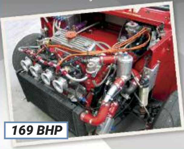
Stage 5 - (5 port) Cylinder Head 37.5mm inlets & 31mm exhaust valves
